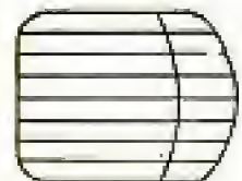
BUCKET SEATS MADE FROM TWO BLOCKS OF PINE GLUED TOGETHER. MARK OFF PLEATS AND CARVE ACCORDING TO SECTION A-A
